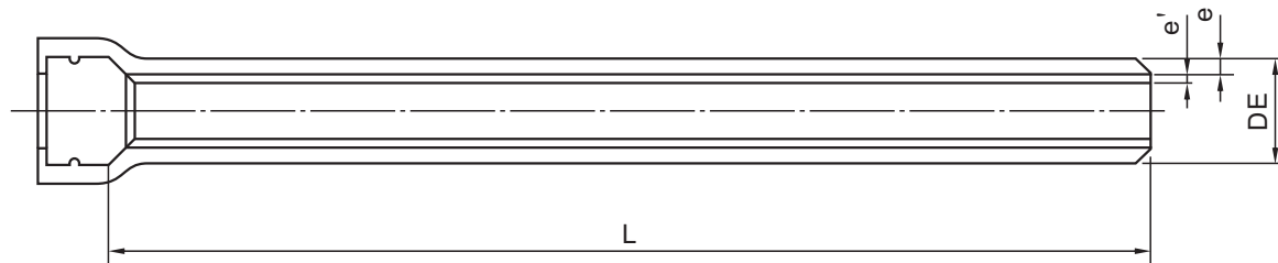
Dimensions of pipes thickness
